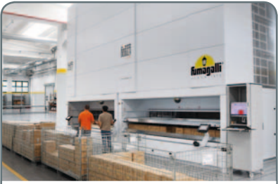
new automated Vertical Warehouse
